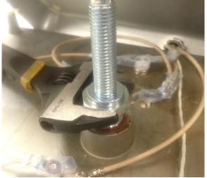
Screw new Adjustment Spindle Bushing into Heater using Crescent Wrench
