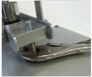
Install Heater by threading Adjustment Spindle into Adjustment Arm using Pliers
