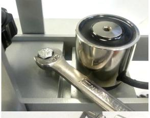
Install Safety Bolt using 1/2" Wrench
