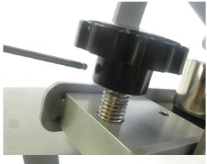
Install pressure adjustment knob by tightening 1/4"-20 x 1/4" set screw using 3/32" Hex Wrench
