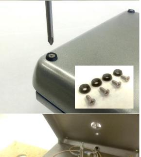
Unscrew 4x #10-24 x 5/8" Screws with Plastic Finishing Washers using #2 Philips Screwdriver
