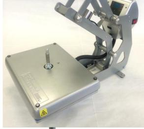
Unthread Adjustment Spindle from Adjustment Arm using Pliers and set down Heater onto Lower Platen
