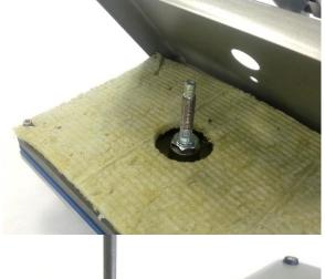
Replace Mineral Wool Insulation as shown and close Heater Cover
